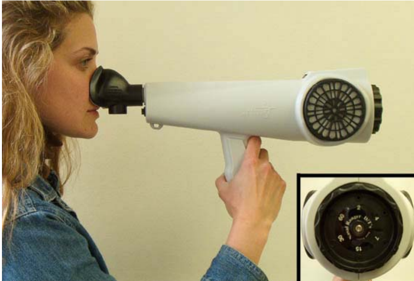
Figure 1 -The Nasal Ranger® Field Olfactometer (St. Croix Sensory, Inc.). The inset picture shows a close-up of the orifice dial, which is located to the right side of the Nasal Ranger in this photo.
