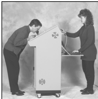
Figure 4. Assessor (left) sniffing from dynamic dilution olfactometer. Photo courtesy St. Croix Sensory, Inc.
