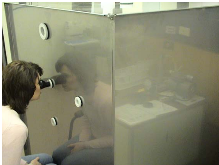
Figure 3. Example small chamber with assessor sniffing directly through the sniffing port. Photo courtesy St. Croix Sensory, Inc.
