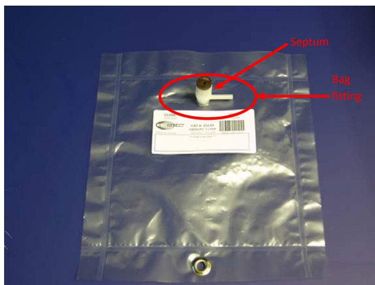
Figure 1. Photograph of 1L Tedlar Bag with Polypropylene Fitting and Septum Assembly
